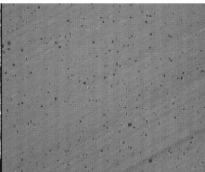
Electron microscope picture of an Ezee cylinder wall after the same friction test: Almost no wear.
