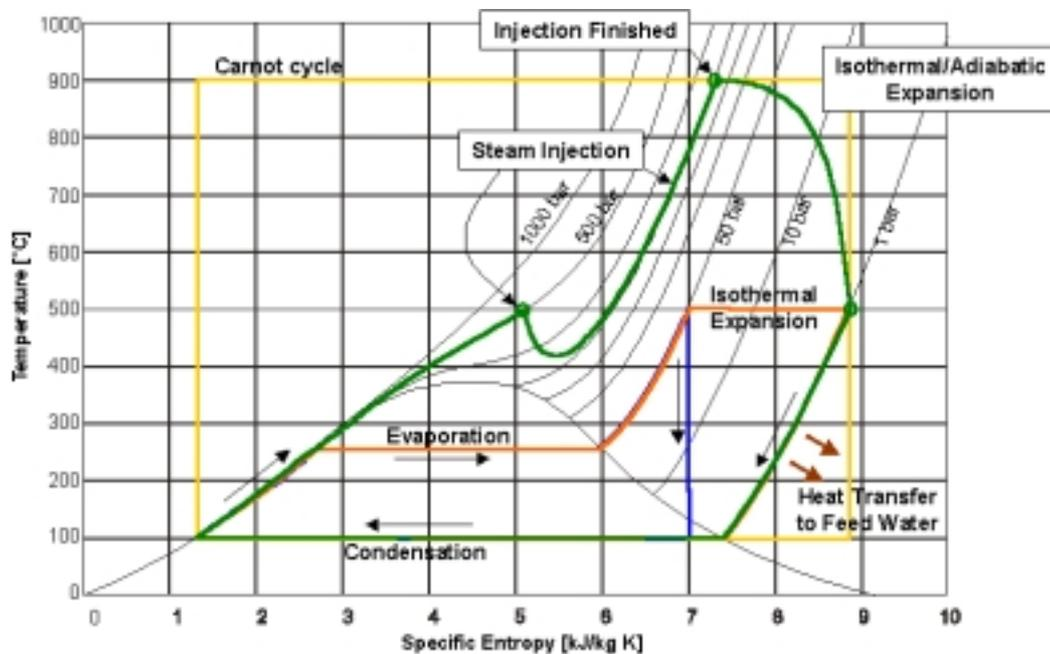
Thermodynamic cycles: A traditional „Rankine cycle steam engine“ passes a wet steam area (evaporation), takes on more heat and finally expands (blue line). The Ezee instead approximates isothermal expansion that is considerably more energetic and efficient (red line). With steam injection system the Ezee’s efficiency could additionally be improved (green line).
