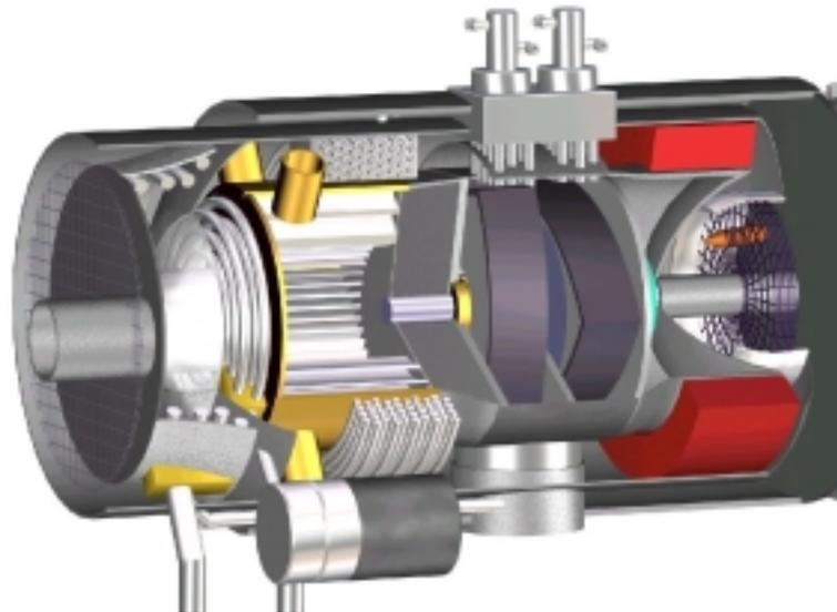
The Ezee Technology allows for large freedom regarding engine layout and design. Shown is an Ezee based drive system with rotary expanders. There is no crankcase necessary.
