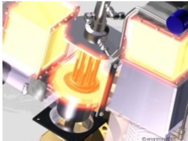
The superheater unit is located between injector and piston. It is directly fired by a CPS Cell.
