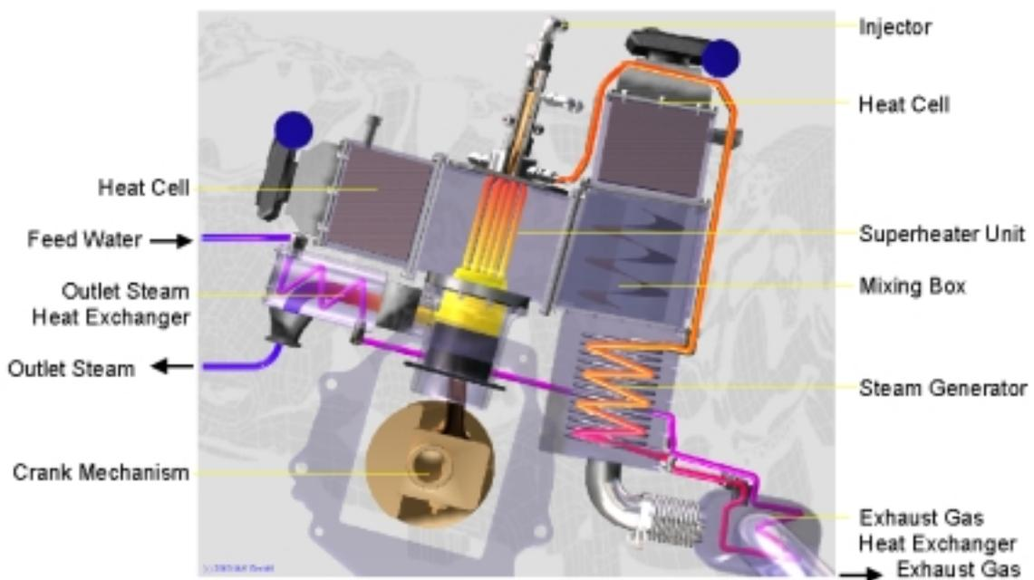
Cross sectional picture of the original research engine that served as component carrier during the Ezee's basic development. It is a 3 cylinder 2-stroke engine with 1 litre displacement. With its compact dimensions it would easily fit under the hood of a compact car. Nevertheless, this engine reaches an incredible torque of up to 500 NM (400 ft.lbs.) – more than conventional V12 engines.
