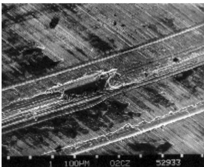
Electron microscope picture of a good commercial dry friction material: Visible scratches.
