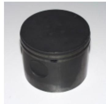
Resulting carbon based piston with carbon based piston rings.
