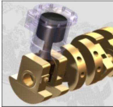
Water lubrication for the research engine's piston, liner and crankshaft bearings.
