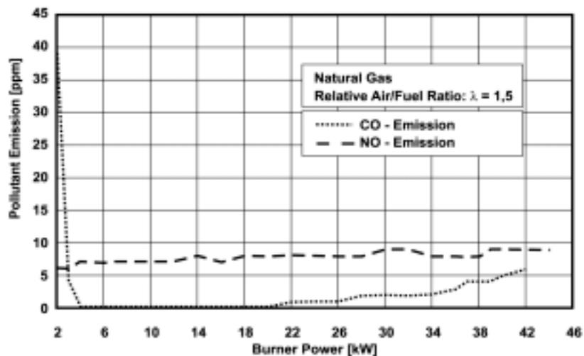
Emissions characteristics of a CPS Cell: Pollutant levels are at the limit of measurability. Hydrocarbons (HC) can not be detected at all. Latest Cell generations achieve another 50% cutback.
