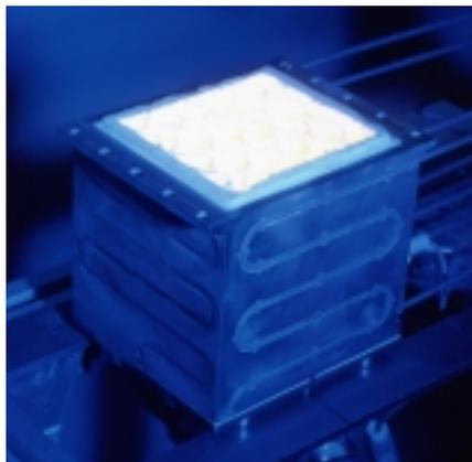
A CPS Cell at full load. Pure thermal energy, no open flame.
