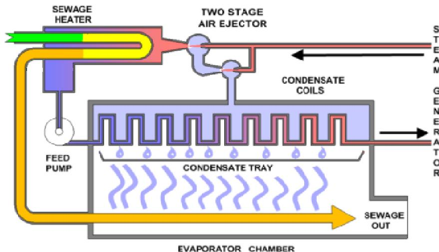
The intertwined steam and water paths serve to minimize the energy expended to evaporate the water in a few different ways. Ejector produced vacuum reduces the evaporating heat requirement, this heat derived from the ejector itself. The condensed ejector discharge is reheated by the evaporated water, returning some of the heat lost in evaporating; the act of condensing causes pressure to drop in the chamber, reducing the amount of steam used by the ejector.
