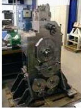
gasoline, diesel and alternative fuels such as CNG and H<sub>2</sub>. All of the FEV Single Cylinder Engines are characterized by a modular architecture and a very robust yet flexible structure, to serve as the basis for a variety of engine set-ups. The main modules are:
