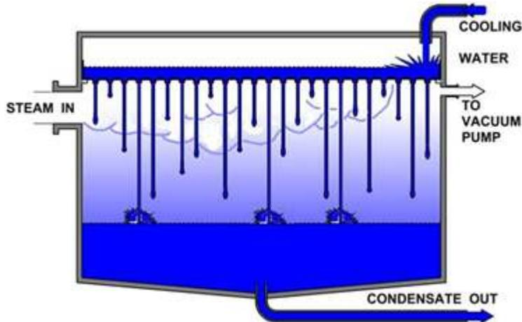
Air-cooled condensers have usually been of the direct contact variety, and almost invariably have been troublesome, but water cooling depends upon a secure water supply. I propose a two-step process: steam will be condensed in a direct contact device, the condensate and entrained steam will then descend through a heat exchanger and be cooled by the air. The two step process appears favorable because compared to steam; water is a superior thermal conductor and better suited to transfer heat.
